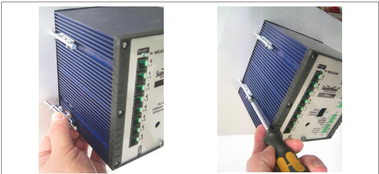
Figure 2.7. Installation of the fasteners
